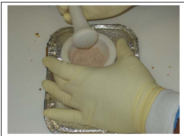
Figure 14. Grind samples into a fine powder, making sure that the sample never thaws. Be careful when pouring liquid nitrogen into the mortar with granulated sample, as the liquid will sometime splash the sample out of the mortar and onto the bench.
