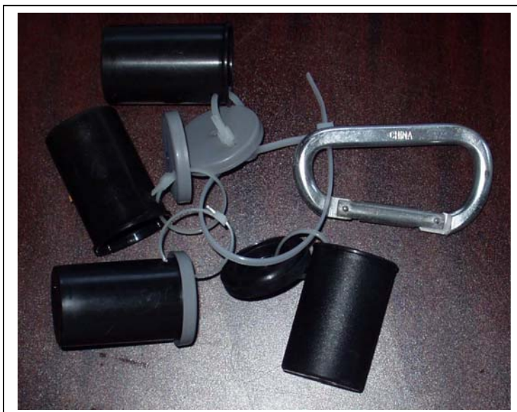
Figure 1. Basic configuration design of 35 mm film canister loop for coral sampling
