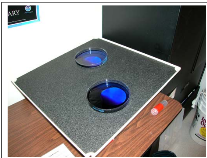
Figure 20. Incubate the filter paper in an incubation boat. The boat can be anything: e.g., petri dish or weigh boat, and be made from plastic or glass. Stain solution should cover the filter paper either in its entirety or so that each rocking slant covers at least 50% of the filter paper in the Stain Solution.
